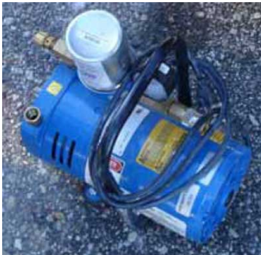
Figure 4. Air pump that supplied breathing air to the supplied air respirator system
